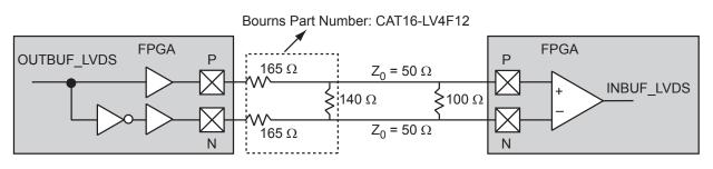
Figure 2-12 • LVDS Circuit Diagram and Board-Level Implementation
