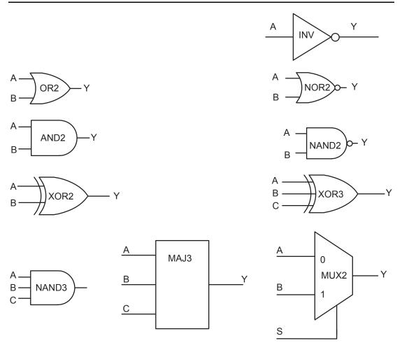
Figure 2-24 • Sample of Combinatorial Cells
