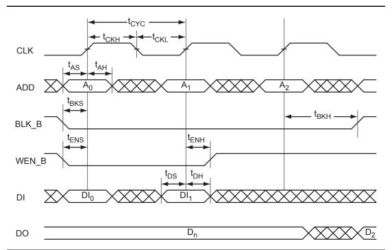
Figure 2-33 • RAM Write, Output Retained (WMODE = 0)
