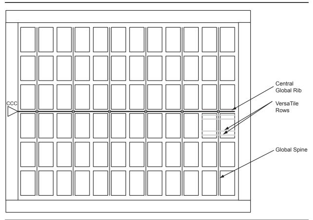
Figure 2-28 • Example of Global Tree Use in an A2F200 Device for Clock Routing
