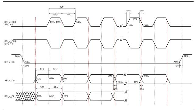
Figure 2-47 • SPI Timing for a Single Frame Transfer in Motorola Mode (SPH = 1)
