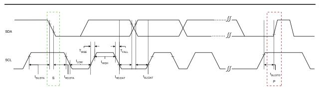
Figure 2-48 • I2C Timing Parameter Definition
