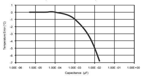
Temperature Error Versus External Capacitance
