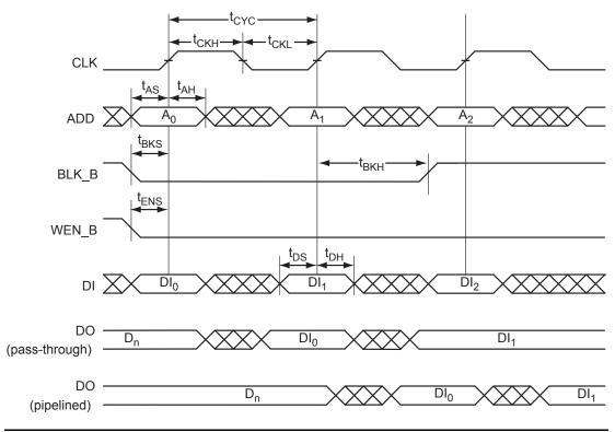
Figure 2-34 • RAM Write, Output as Write Data (WMODE = 1)
