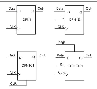
Figure 2-26 • Sample of Sequential Cells
