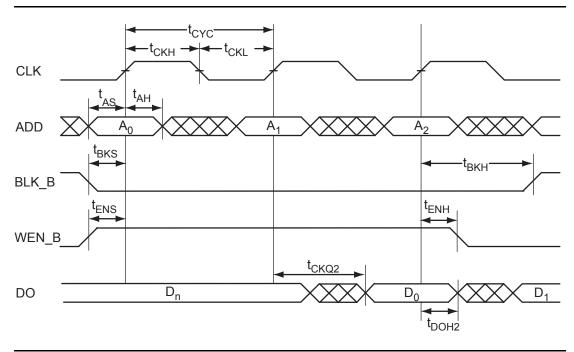
Figure 2-32 • RAM Read for Pipelined Output
