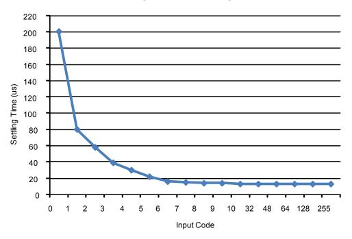
Figure 2-44 • Sigma-Delta DAC Setting Time
