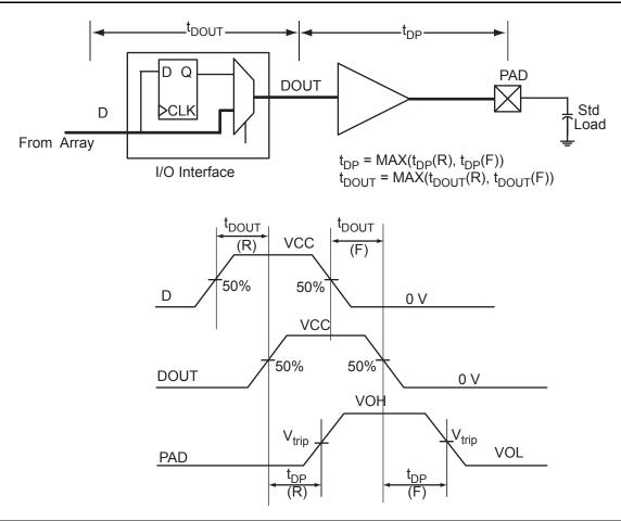
Figure 2-5 • Output Buffer Model and Delays (example)
