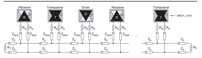
Figure 2-13 • B-LVDS/M-LVDS Multipoint Application Using LVDS I/O Buffers
