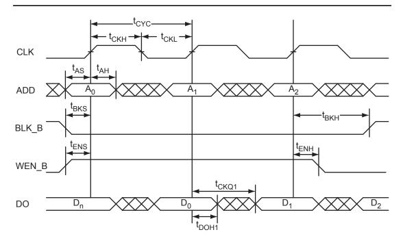
Figure 2-31 • RAM Read for Pass-Through Output
