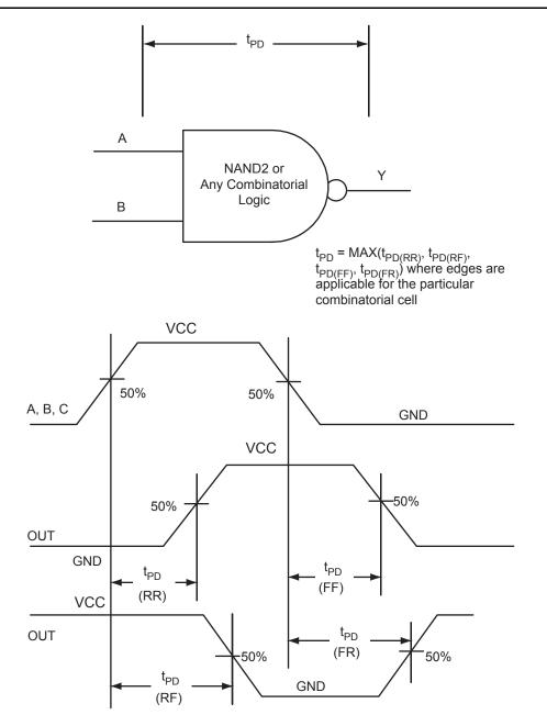
Figure 2-25 • Timing Model and Waveforms
