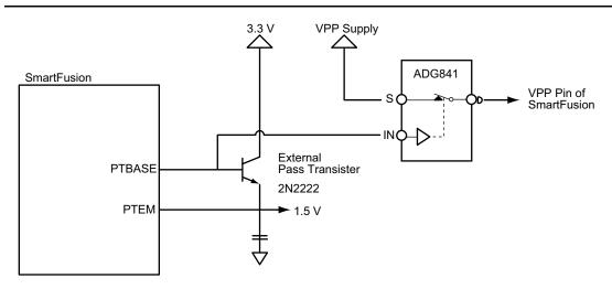
Figure 2-2 • Implementation to Control VPP
