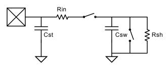
Figure 2-43 • ADC Input Model
